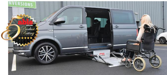
The Transporter can be configured for rear or side entrance, for drive from wheelchair or upfront passenger purposes (with flattened floor) as well as internal transfer – and is tested for wheelchairs up to 200kg. They also feature inboard or under floor lift options.
