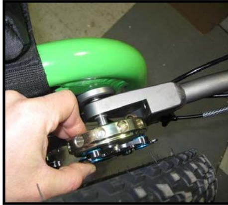
3. Slide Drive unit onto pivot pin – make sure it is the correct drive unit for that side of the trike. Check this by rotating the gold engagement ring (with holes in).
