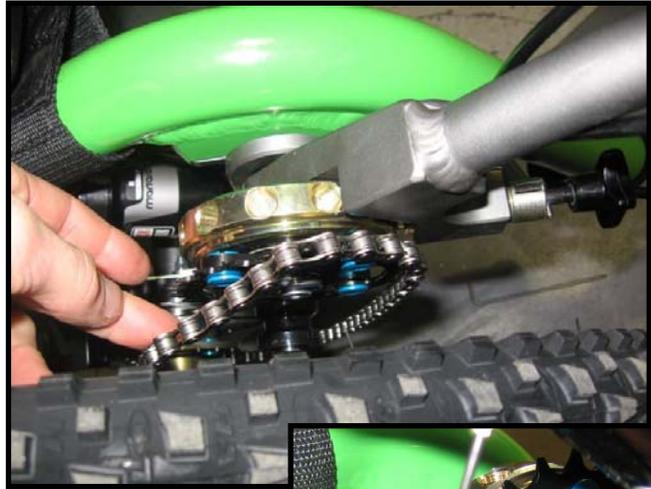
6. Remove the end bolt to allow the drive unit and gear to slide off. \* **there is a small centre spacer between the drive unit and the drive lever which may stick to the drive unit when removed\***
