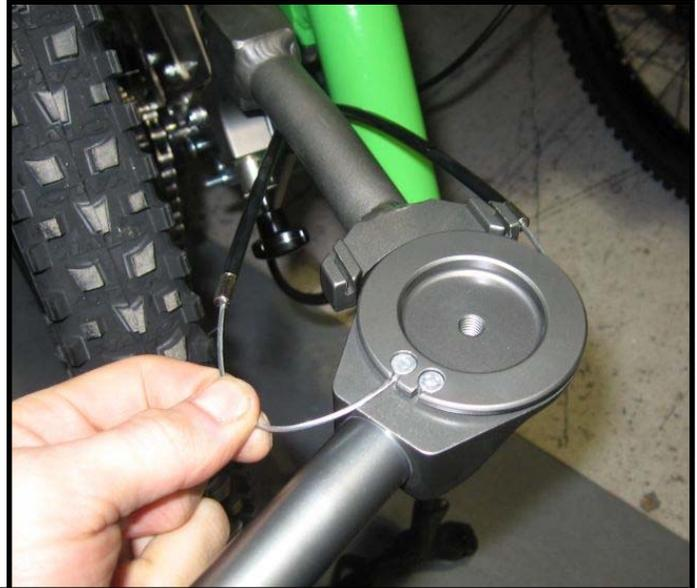
13. Slide drive lever off pivot pin **\*there is a small spacer between the drive lever and swingarm, make sure this stays in place, there is no need to remove it\***
