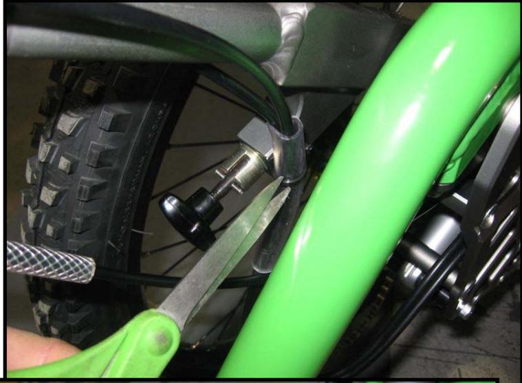
9. With 4mm allen key loosen steering cable tension bolts and pull cable slack
