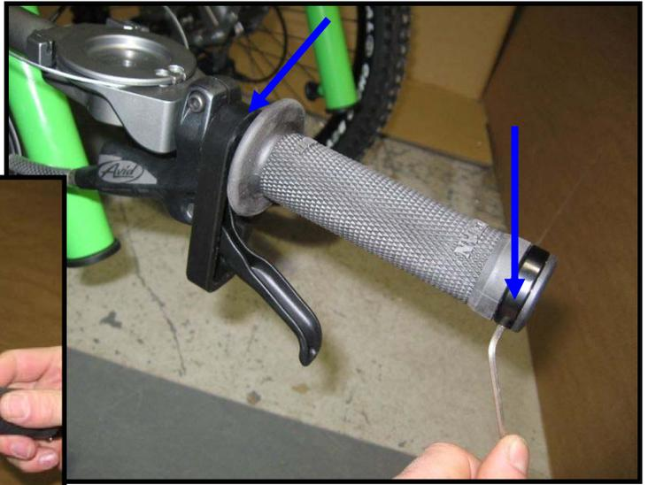
11. Undo brake lever with 4mm allen key and slide off with parking brake
