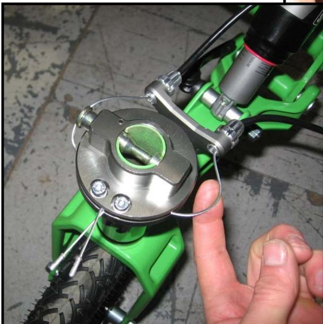
10. Undo upper and lower Hand Grip collars with 2.5mm allen key and slide grip off
