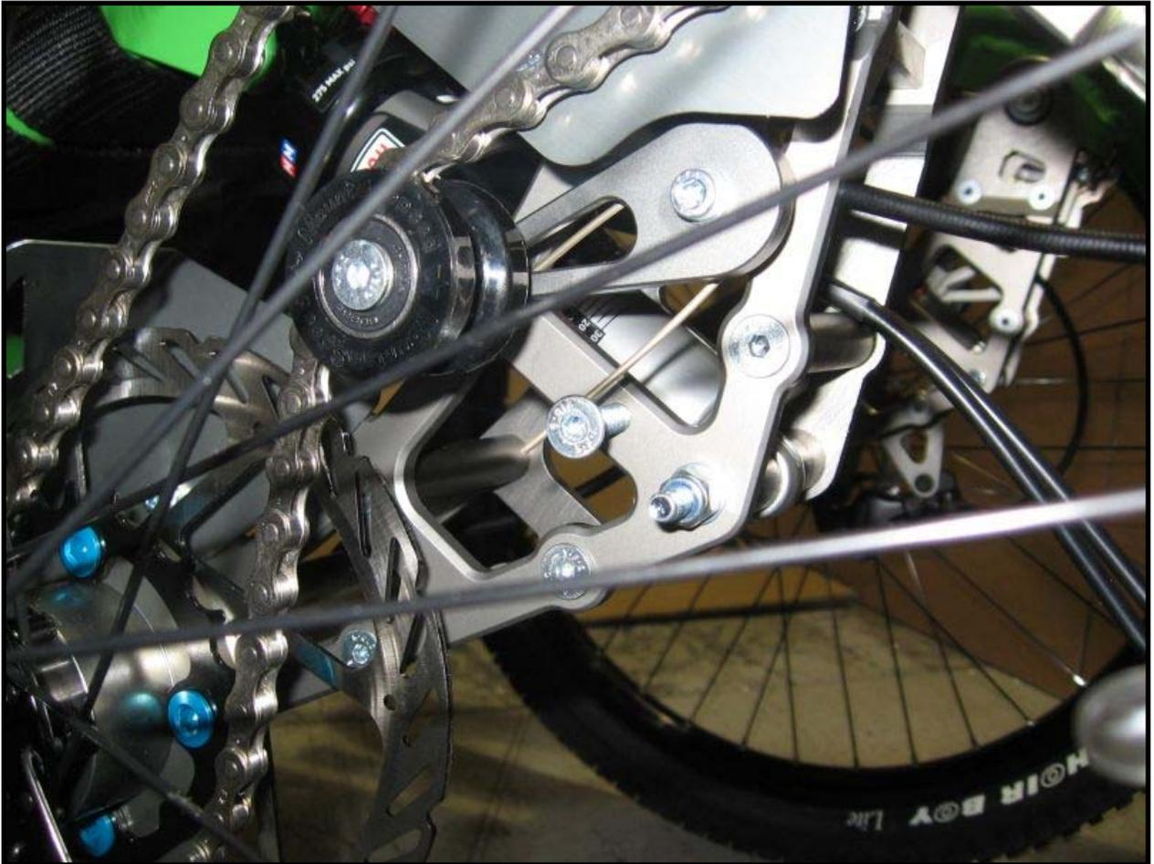
8. Lift wheel off the ground and spin it to check the chain spins freely and that drive engages correctly.
