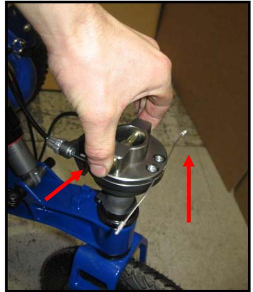
2. Compress headset/fork assembly and tighten Fork Clamp with 4mm allen key.
