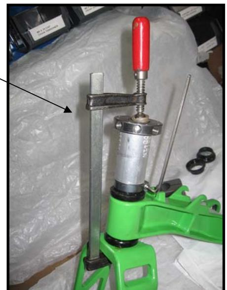
3. Slide Steering unit back onto fork by compressing Quick Release pin and locating in slot securely
