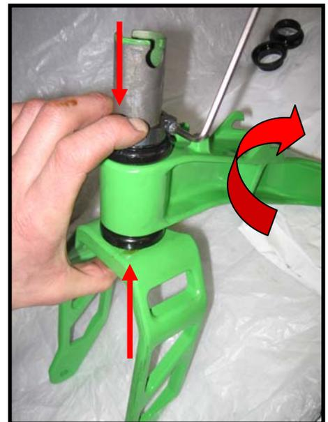
Also, you may find it easier to use a clamp and piece of tube to compress the bearings before tightening.
